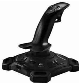
Figure 6. Joystick Attack 3 issues commands via USB
