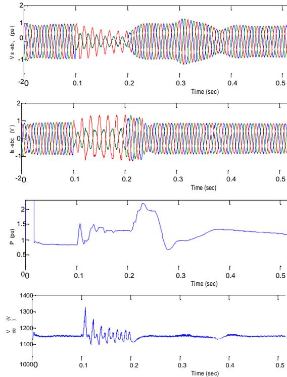
Figure 9.  $V_s$ ,  $I_s$ ,  $P_s$ ,  $V_{dc}$  with the proposed control strategy for the RSC and GSC when the phase A and phase B to ground fault
