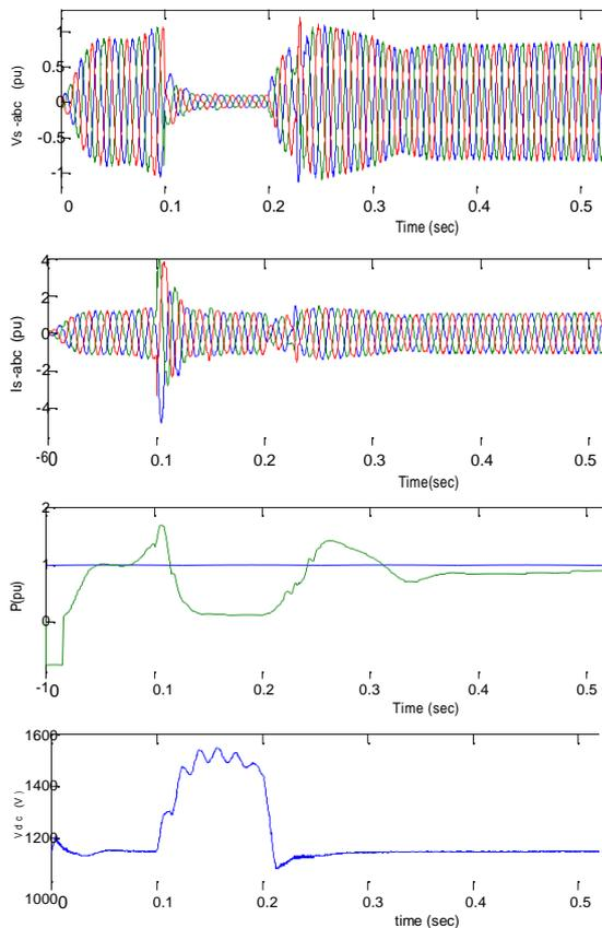
Figure 8.  $V_s$ ,  $I_s$ ,  $P_s$ ,  $V_{dc}$  with the proposed control strategy for the RSC and GSC when the three-phase to ground fault
