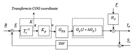
Figure 2. Closed loop control diagram with power amplifier dynamics, system uncertainty, imbalance disturbance and sensor noise
